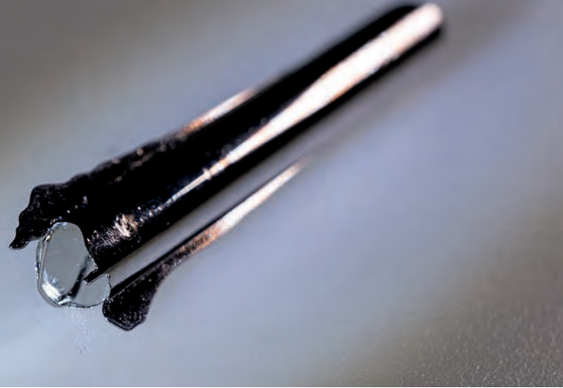
Metallic glass looks like an ordinary metal from the outside. On the inside, however, it lacks a crystalline lattice structure. This makes it strong and brittle. · Photo: Jens Meyer
