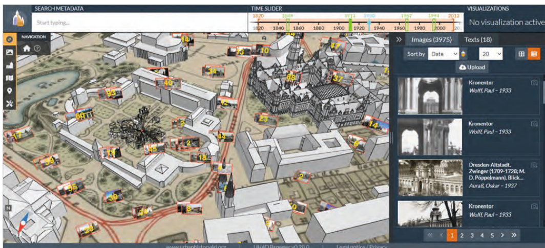
Interface of the »4D Browser« web application. Historical photographs are precisely located in a 3D urban model. The section shown here depicts the Old Town of Dresden, complete with the Zwinger complex and the Royal Palace. The project team includes researchers from the University of Jena, the University of Würzburg, Bielefeld University, LMU Munich and Cologne University of Applied Sciences.
