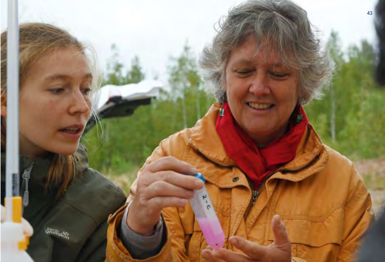
Lisa Schulz (left), a bachelor's student in Biogeosciences, and Prof. Erika Kothe discuss the samples that are titrated to measure soil respiration. The phenolphthalein dye turns from pink to colourless when the pH becomes neutral. This is how the researchers can measure how much CO 2 the microorganisms have produced.
