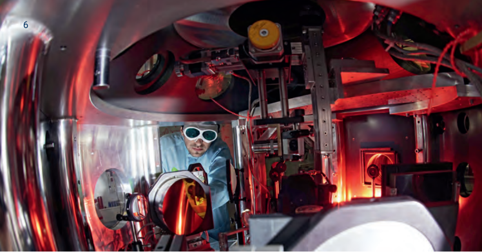
Nonlinear optics research laboratory: a target chamber of the »Jena Titan: Sapphire 40-Terawatt Laser Systems« or »JETI40« for short.
