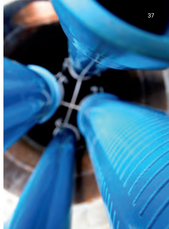
Measuring tube of a groundwater well, used for various purposes, such as taking groundwater samples, monitoring probes or on-site experiments.
